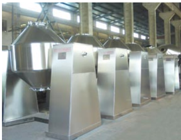
◆ 双锥回转真空干燥机制作现场。 ◆ Manufacturing site of SZG Series Conical Vacuum Dryer
